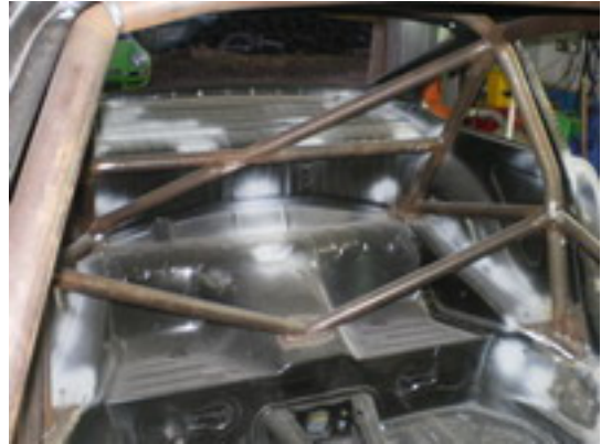
Full custom built, FIA approved welded in roll cage
