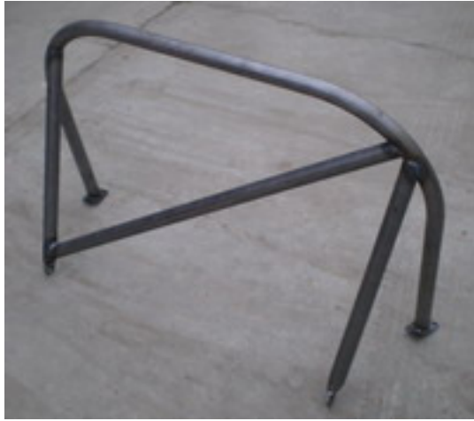
ST style rear cage before being powder coated
